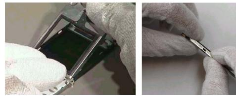
10. Fit the Display Shield in its place.
