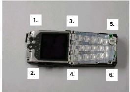
15. Tighten the six screws by using following order.
