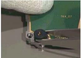
12. Put the Microphone into the frame.
