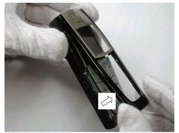
2. Flip gently the A-cover from down corner. Remove the A-cover.
