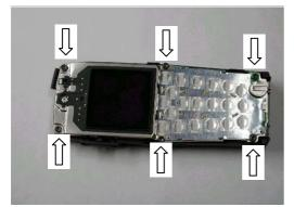
7. Remove the screws (6pcs) to get the module out from C-cover.
