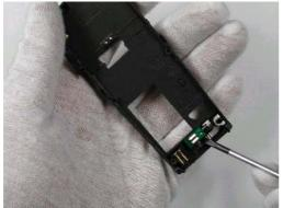
16. Remove the Vibra by lifting it out of its place.
