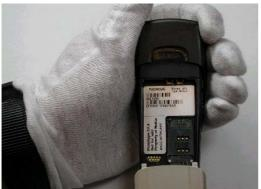
19. Slide the Battery cover into its place until the Release Key locks it.
