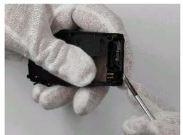
17. Remove the DC Jack by lifting it out of its place
