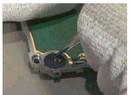
10. Remove the microphone by pressing it from its edge, or take the tweezers between the frame and microphone and lift it out from the frame.
