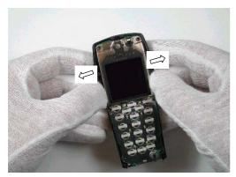
4. Spread the B-cover from both sides until snaps inside will release it.
