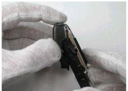
16. Place the B-cover into its place. Make sure the snaps on both sides are locked to the module.
