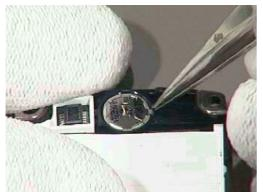
11. Remove the speaker by lifting it from the guiding pin.
