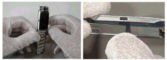
12. To remove the Display shield, open the snaps from both sides by using the specified tool and remove the shield.
