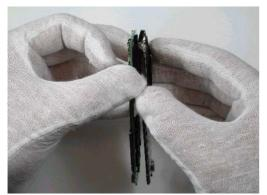
9. Remove the UI module from the engine board.
