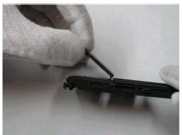
7. Put the Antenna into its place
