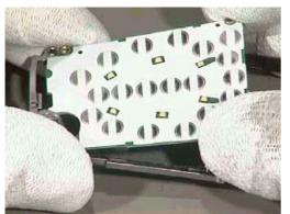
14. Remove the UI Board from the LCD frame.
