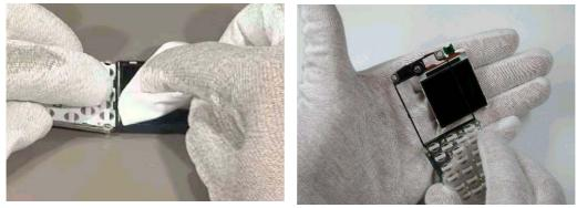
13. To remove the LCD Module, keep it on a table by using soft cloth, and flip the LCD frame <u>gen-</u><u>tly</u> until the LCD Module detaches.
