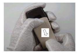
1. Place the phone face down, press the Release Key and slide the battery cover downwards.
