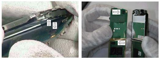
NOTE! The UI module and the engine board are linked together by two board-to-board connectors. Be careful not to damage them.
