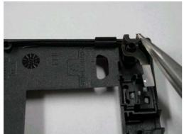
18. Lift the Release Spring by tweezers from its place
