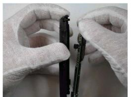
8. Remove the module out from the C-cover.
