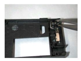
2. Put the Release Spring into its place.
