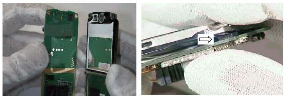
13. Place the UI Module and the engine together by closing the Display connector.
