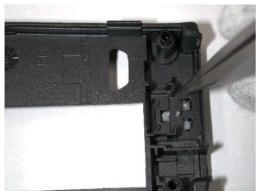
19. Remove the Release Key by pressing the snaps towards the center from inside.
