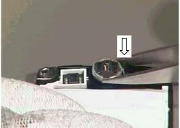
11. Put the Speaker into the frame so that the guiding pin goes into its place.
